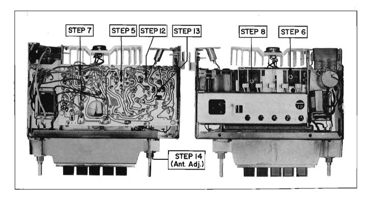
Figure 34 - ALIGNMENT PROCEDURE - ALL MANUAL RADIOS
