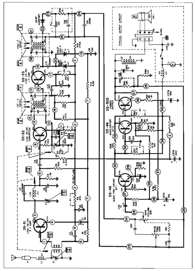
CIRCUIT DIAGRAM - 986096-986201-986248-986113-986330-986338-986339 - PASSENGER CAR AND TRUCK MANUAL RADIOS 3 Figure
