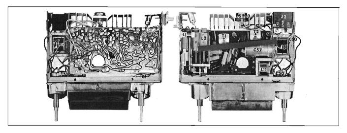
Figure 37 - CHEVROLET PARTS LAYOUT CIRCUIT BOARD VIEW - 986096 RADIO
