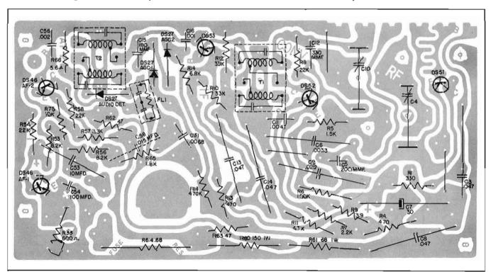
Figure 29 - PARTS LAYOUT ON CIRCUIT BOARD - ALL MANUAL - RADIOS
