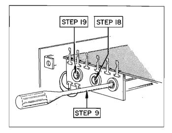
Figure 33 - CORE ADJUSTMENTS
