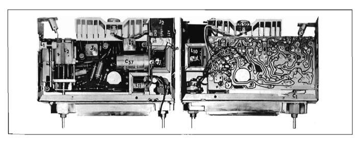
Figure 47 - CORVAIR 95 PARTS LAYOUT - CIRCUIT BOARD VIEW - 986330 - RADIO
