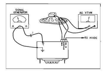
Figure 32 - HOOK-UP FOR SIGNAL AND OUTPUT METER
