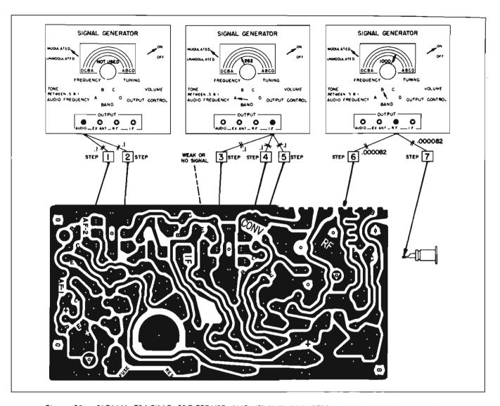
Figure 30 - SIGNAL TRACING PROCEDURE AND ISLAND NUMBERS - ALL MANUAL - RADIOS
