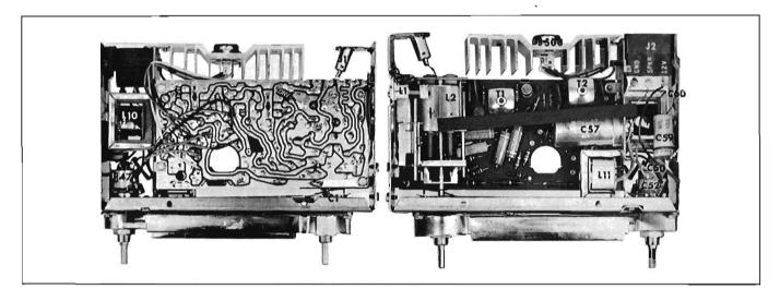
Figure 45 - CHEVROLET TRUCK - PARTS LAYOUT - CIRCUIT BOARD VIEW - 986338 - RADIO
